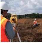
Multi Pulse optical system contributed to power consumption cut down from 4.7W to 3.6W (±20% down), but extended operating time to 5 hours (+120%)
