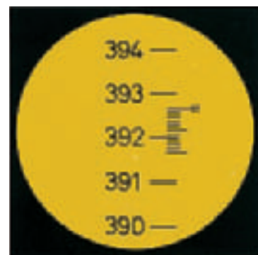
NAK2 circle reading (400 gon) 392.66 gon
