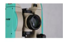
300m distance measurement with Prism, with 3mm+2ppm distance accuracy.
